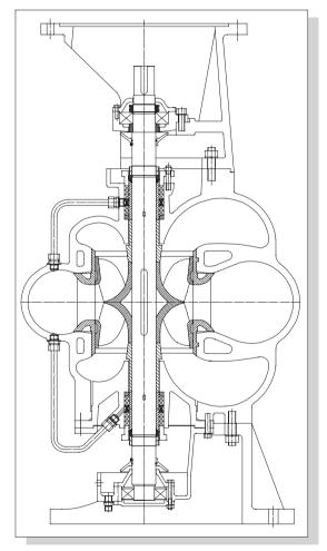
Suction and discharge flanges are located at an angle of 180° to each other. Impeller is double-entry. Shaft seal: packing seal or mechanical seal. Electric motor is mounted on the top of the pump. If required, it can be mounted with the help of extension shaft.
